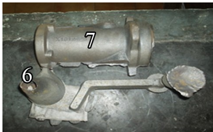
Fig. 8. Casting with redesigned gating and risering systems
