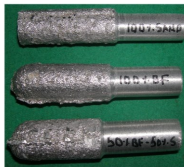
Fig. 1. A 356 alloy finished cylindrical castings before and after machining
