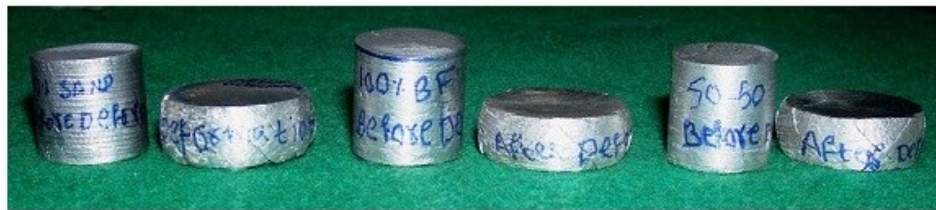
Fig. 4. Cylindrical samples with aspect ratio = 1.0 showing bulge profiles before and after deformation under compression
