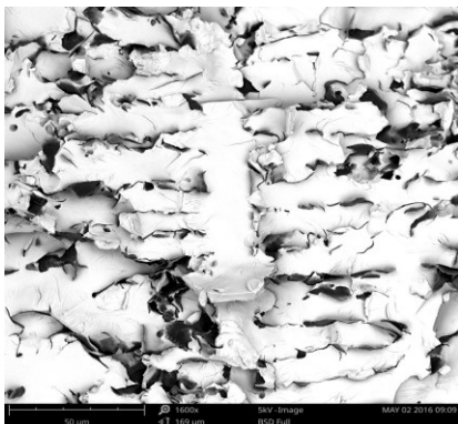
Fig. 5. Fracture of alloy No. 2. SEM.
