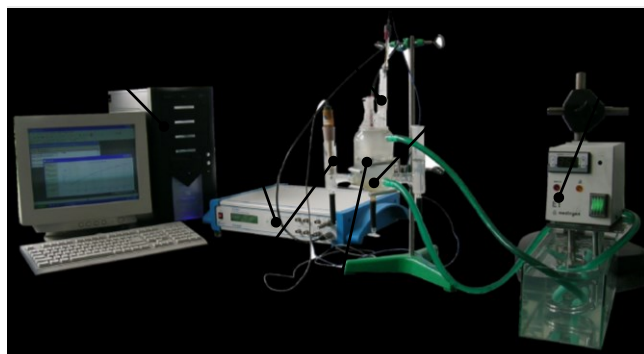
Fig. 3. The measuring set used in the study[14-16]: a – set of recording graphs anodic polarization curves, b – potentiostat VoltaLab® PGP201, c – reference electrode - impregnated calomel electrode (NEK) type KP-113, d – electrochemical cell test, e – thermostat Medlingen, f – secondary electrode – platinum electrode type PtP – 201, g – anode - test sample
