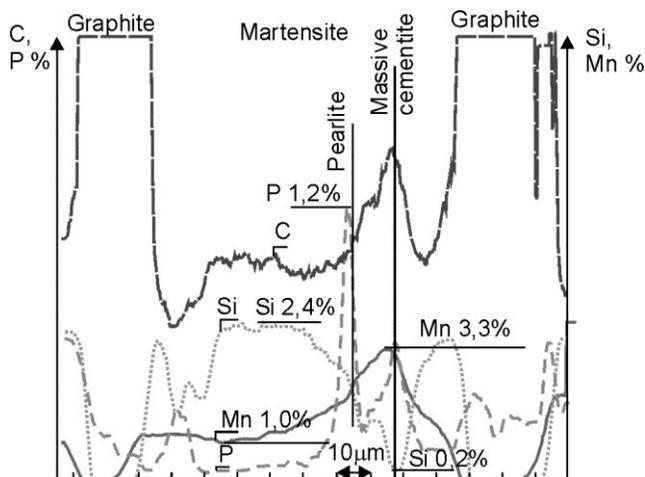
Fig. 15. Distribution of C, Mn, Si, and P in a sample of cast iron austenitized at 900°C and held at 760°C over 120s
