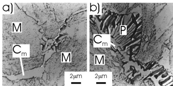
Fig. 4. Micrograph of cast iron austenitized at 1020°C and held at 820°C, duration (a) 60s, (b) 240s, TEM imaging
