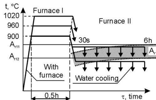
Fig. 2. Diagram of the CI heat treatment
