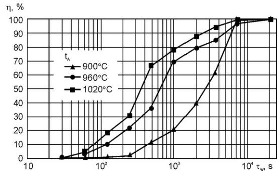
Fig. 12. Overall degree of eutectoid reaction  $\eta$  for the cast iron during isothermal holding at 760°C
