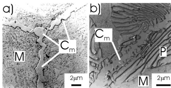
Fig. 7. Micrograph of cast iron austenitized at 1020°C and held at 760°C, duration (a) 30s, (b) 240s, TEM imaging
