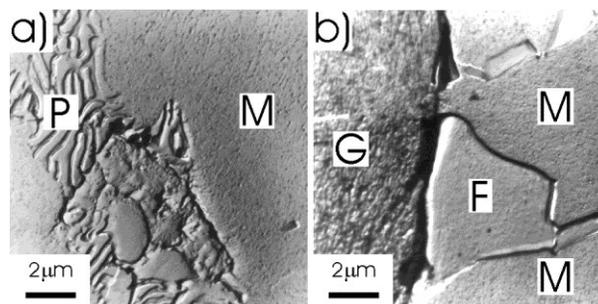
Fig. 6. Micrograph of cast iron austenitized at 900°C and held at 760°C, duration (a) 120s, (b) 240s, TEM imaging, two-stage carbon replica
