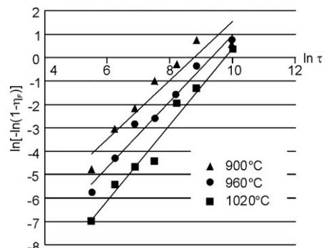
Fig. 13. Ferrite content vs. cast iron isothermal holding time at 760°C
