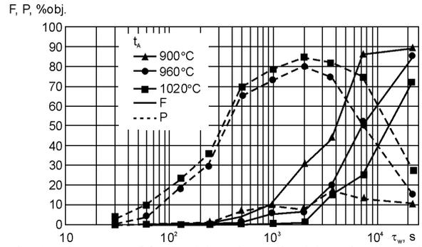
Fig. 11. Contents of ferrite (F) and pearlite (P) vs. isothermal holding time at 760°C of the cast iron austenitized at 900, 960 or 1020°C
