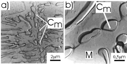
Fig. 8. Micrograph of cast iron austenitized at 1020°C and held at 760°C, duration 960s: (a) lattice fragmentation, (b) spheroidization of network fragments, TEM imaging
