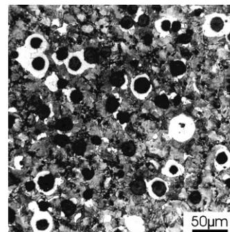
Fig. 1. CI structure, as cast, nital etched, LM
