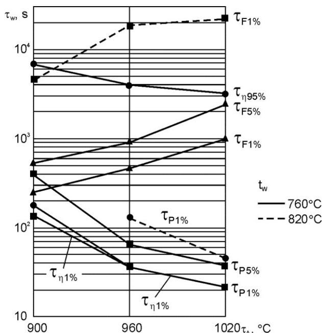
Fig. 14. Time required to achieve the specific transformation phase as a function of austenitizing temperature
