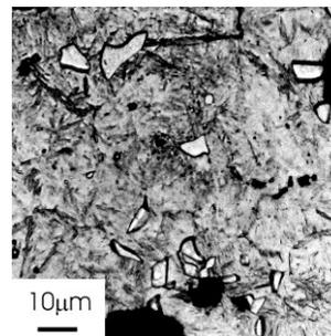
Fig. 5. Micrograph of cast iron austenitized at 960°C and held at 820°C, duration: 6 h, nital etched, LM
