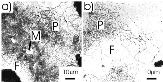
Fig. 9. Micrograph of cast iron austenitized at 960°C and held at 760°C, duration (a) 1800s, (b) 6h, LM
