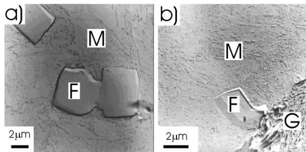
Fig. 3. Micrograph of cast iron austenitized at 900°C and held at 820°C, duration (a) 1800s, (b) 3600s, TEM imaging
