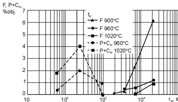
Fig. 10. Contents of ferrite (F), pearlite (P) and networked cementite ( $C_m$ ) vs. cast iron isothermal holding time at 820°C
