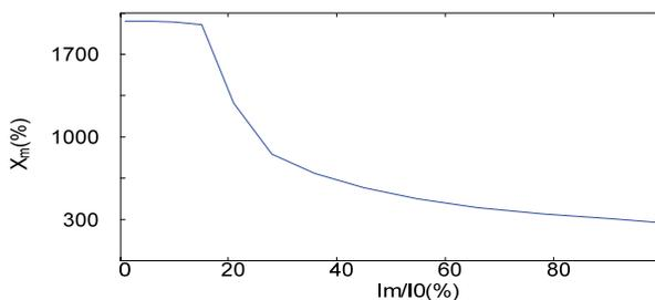
Fig. 7. Nonlinear magnetizing reactance ( $X_m$ )
