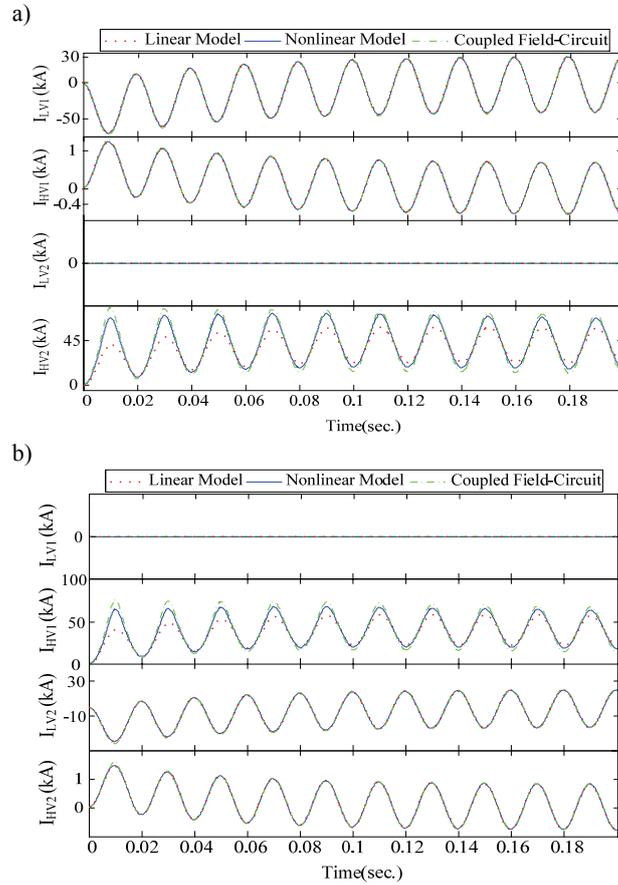
Fig. 13. Inrush and short-circuit currents while a) LV1 or b) LV2 winding is short-circuited (cases III, IV)
