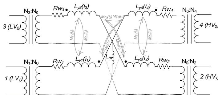
Fig. 8. Novel nonlinear equivalent circuit for split-winding transformer, including magnetizing reactances and windings resistances
