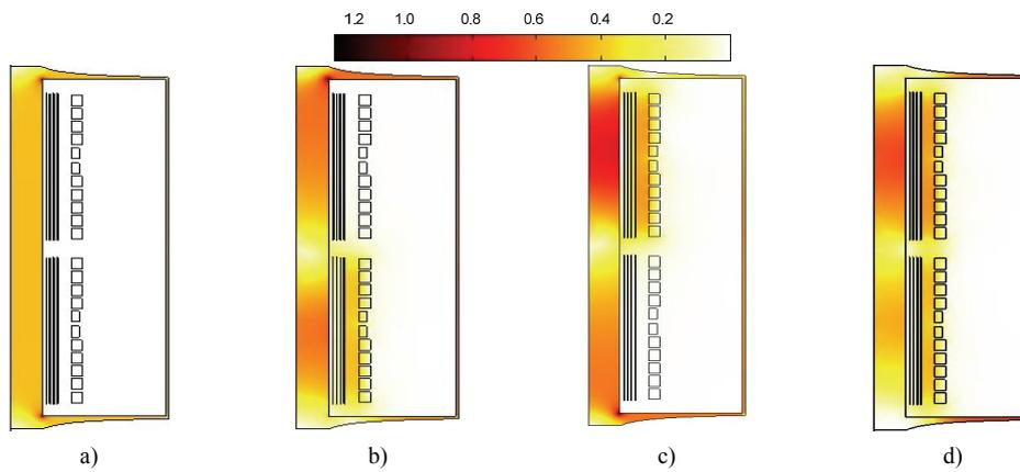
Fig. 14. Magnetic flux density in different loading conditions: cases a) I, b) II, c) III and d) IV
