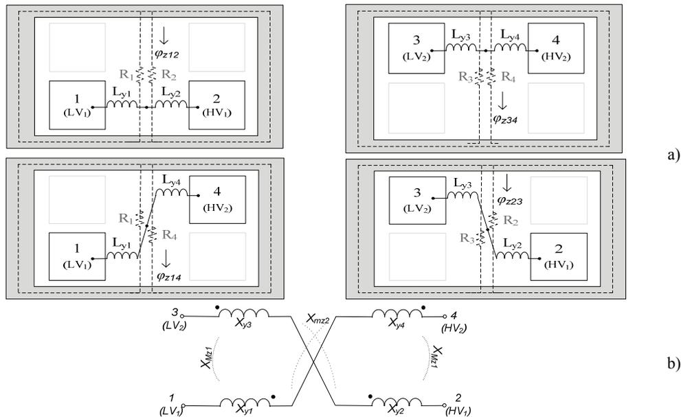
Fig. 2. a) Magnetic circuits represent the axial leakage flux paths and b) final Leakage model of a four-winding traction transformer
