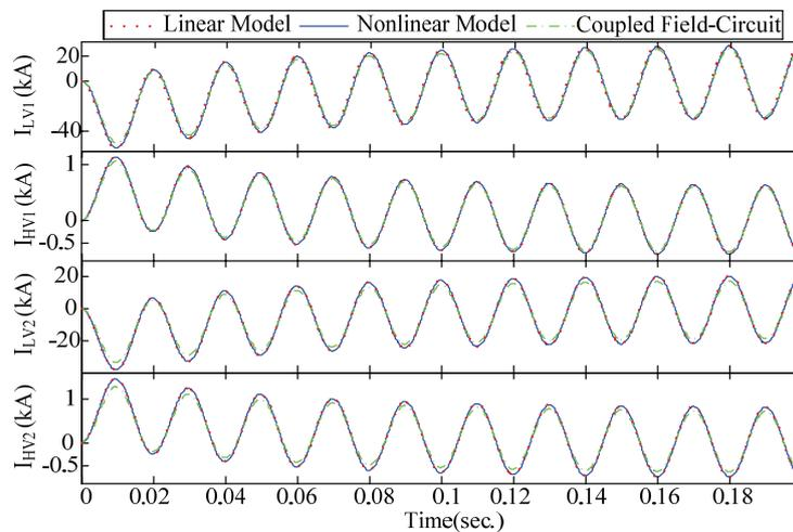
Fig. 12. Short-circuit currents, while both LV windings are short circuited (case II)
