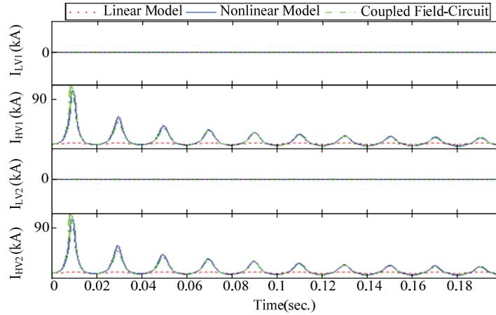
Fig. 11. Inrush currents, while both LV windings are open circuited (case I)
