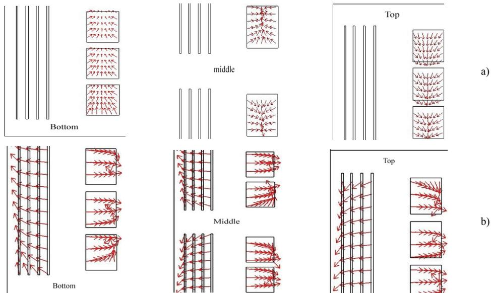
Fig. 15. Electromagnetic force distribution in bottom, middle and top of windings due to a) no-load and b) short-circuit conditions
