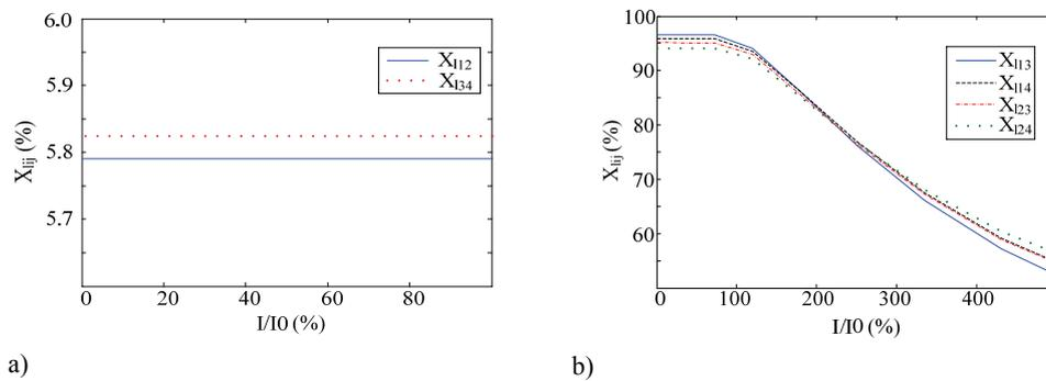
Fig. 5. Nonlinear reactances of a) concentric and b) pancake windings in the split-winding transformer
