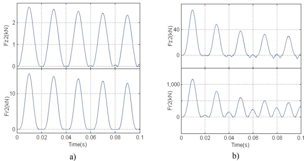
Fig. 16. a) Inrush and b) Short-circuit forces in bottom high voltage winding (Fz, Fr: axial and radial forces)
