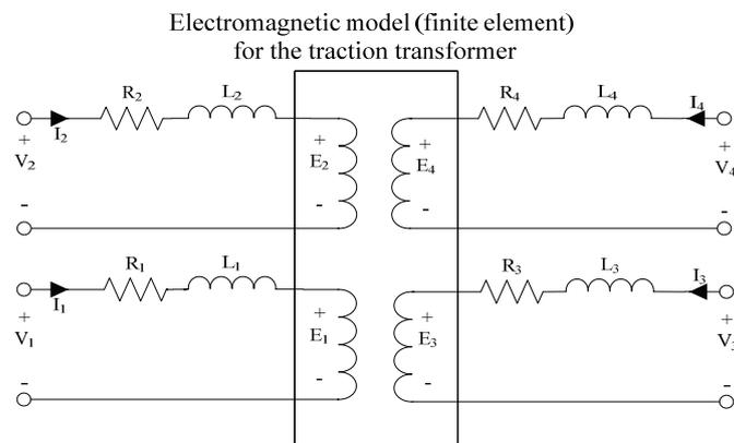
Fig. 9. Schematic view of the coupled field-circuit approach
