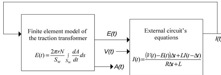
Fig. 10. The coupled field-circuit method
