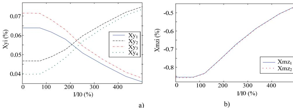
Fig. 6. Nonlinear leakage reactances of the nonlinear star model, a)  $X_{y_i}$ , b)  $X_{mz_i}$
