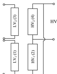
Fig. 1. Schematic view of split-winding transformer
