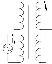
Fig. 3. Short-circuit test for measuring the leakage inductance between a pair of windings
