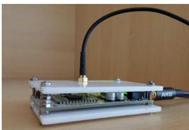
Fig. 3. Operating programmable DAB+ receiver.
