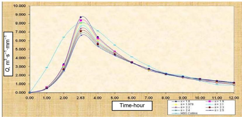
Fig. 5. Comparison between synthetic unit hydrograph of Nakayasu (Nakayasu SUH) with some  $\alpha$  parameter and observed unit hydrograph (HSO); source: own study
