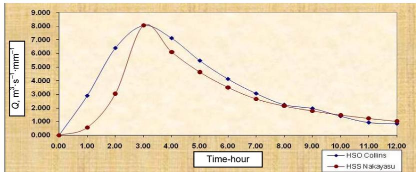
Fig. 6. Comparison between synthetic unit hydrograph of Nakayasu (Nakayasu SUH) with  $\alpha = 1.979$  and observed unit hydrograph (HSO); source: own study
