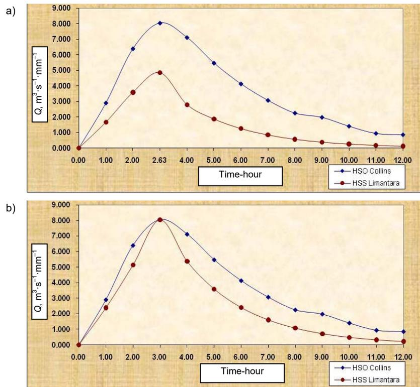
Fig. 7. Comparison between Observed Unit Hydrograph HSO of Collins (HSO-Collins) and synthetic unit hydrograph of Limantara (Limantara SUH): a) before calibration, b) after calibration; source: own study
