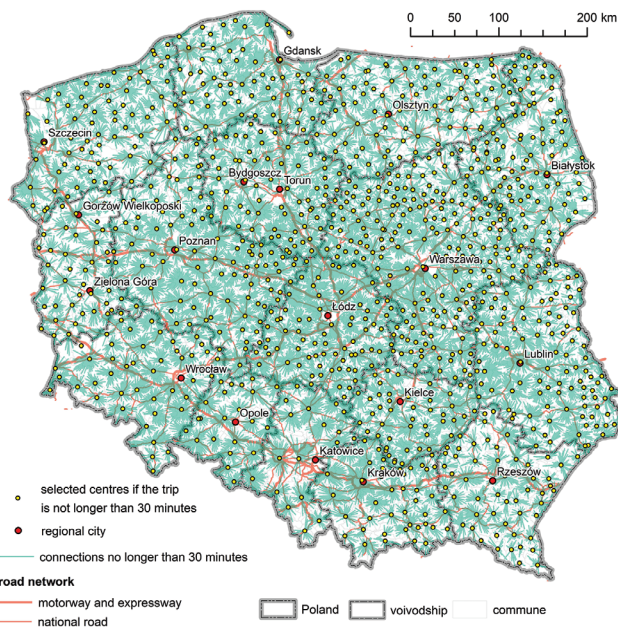
Fig. 2. Optimum distribution of regional centres with the assumption of maximum 30-minute theoretical travel time to all settlement units in Poland
