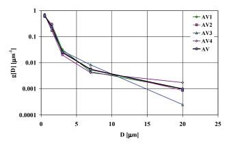
**Fig. 1.** Probability density of the equivalent diameter of dust particles in a sample taken from a disc brake: the average values for individual analysed places (AV1 through AV4) and the average value for the sample as a whole (AV) (Report of project NR10-0050-10 2013)
