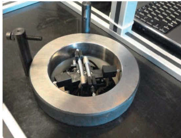
Fig. 6. The gauge head inside the master ring during tests.
