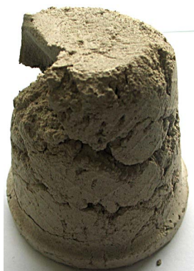
Phot. 4. The solidified sample of drilling-related waste from B-1 opening (binding additive 2.5% SCQ25 + 0.5% of sodium water glass)
