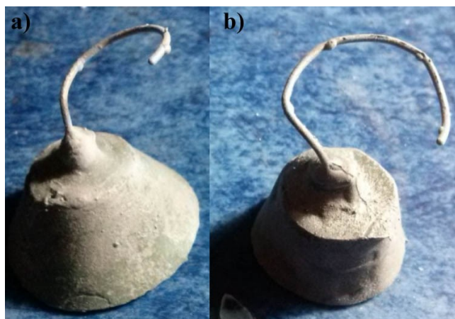
Fig. 1. Spiral test castings of 0,8 mm diameter a) Ceranium NC alloy, b) Magnum AN alloy
