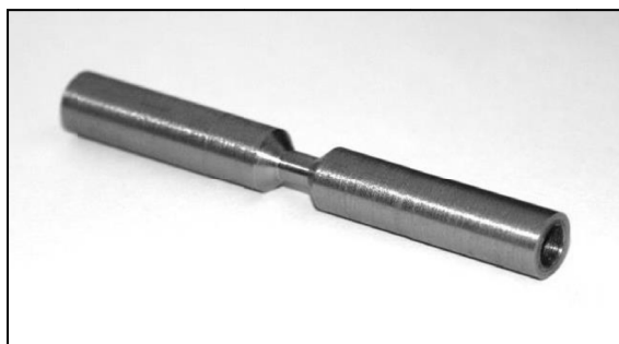
a) Special sample for dilatometric tests without deformation
