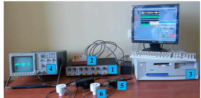
Fig. 1. General view of the measuring system EA DEMA-COMP: 1 – apparatus set of DEMA, 2 – PCI-610E measuring card and CB6-TP measuring terminal, 3 – PC computer, 4 – oscilloscope, 5 – preamplifier, 6 – AE measuring sensor.
