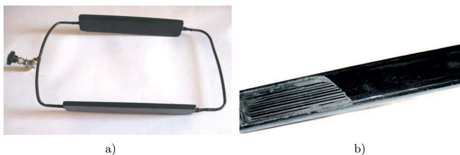
Figure 3: Flat loop thermosyphon made from polymer composite-polyamide reinforced with carbon micro-/nanofilaments and nanoparticles (a) and flat evaporator (cross-sectional view) with rectangular minichannels (b).
