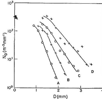
Fig. 1. Curves of Laws and Parsons in a matching with experimental data [26]
