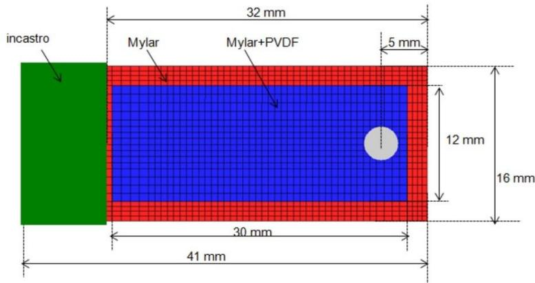
Fig. 11. FEM model of measurement specialties LDT1-028K
