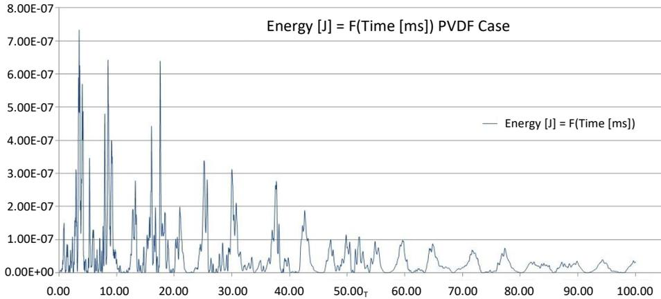
Fig. 16. Electrical energy (J) converted by PVDF patch from an impact with a raindrop with a diameter of 3.3 mm and limit velocity of 8.3 m/s vs time (ms)
