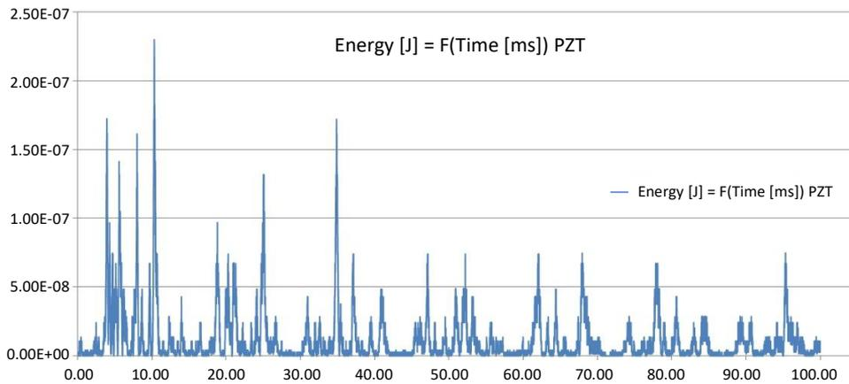
Fig. 18. Electrical energy (J) converted by PZT patch from an impact with a raindrop with a diameter of 3.3 mm and limit velocity of 8.3 m/s vs time (ms)
