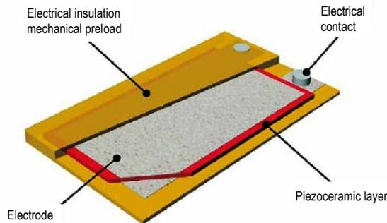
raindrop's impact is modelled with a time history of force applied in the region of impact between the surface of the patch and the raindrop.
