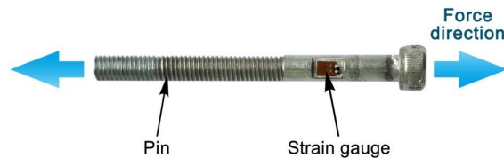
Fig. 3. Pin with foil strain gauge
