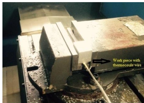
Fig. 2. Work piece mounted on machine with thermocouple
