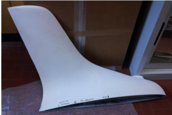
Fig. 1. The investigated composite full scale blended winglet
