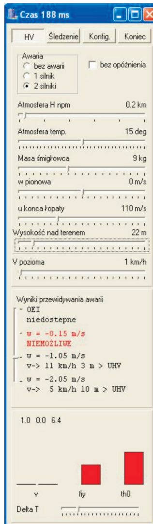
Fig. 22. Form displaying the parameters of flight and predicting the allowable maneuver in the case of engine failure. For the radio-controlled model of helicopter Benzin Trainer, autorotation soft landing with vertical speed w = -0.15 m/s will be impossible.
