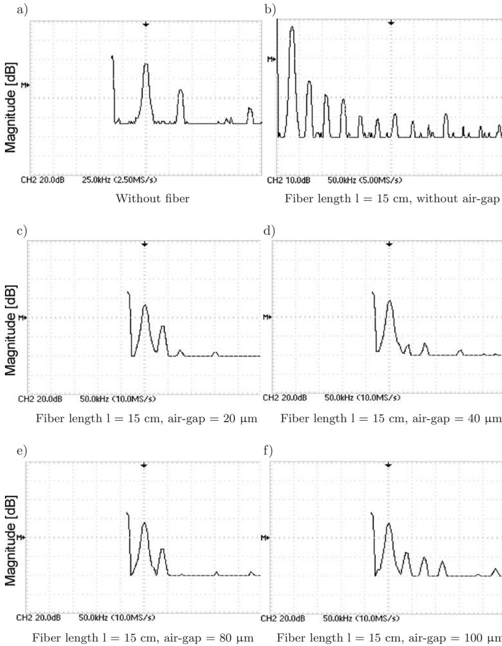
Fig. 6. Ultrasonic output signal spectrum: a) sandwich transducer without a fiber, b) after attaching an optical fiber, without the air gap, c) after attaching an optical fiber with an air gap =  $20 \mu\text{m}$ , d) after attaching an optical fiber with an air gap =  $40 \mu\text{m}$ , e) after attaching an optical fiber with an air gap =  $80 \mu\text{m}$ , f) after attaching an optical fiber with an air gap =  $100 \mu\text{m}$ .
