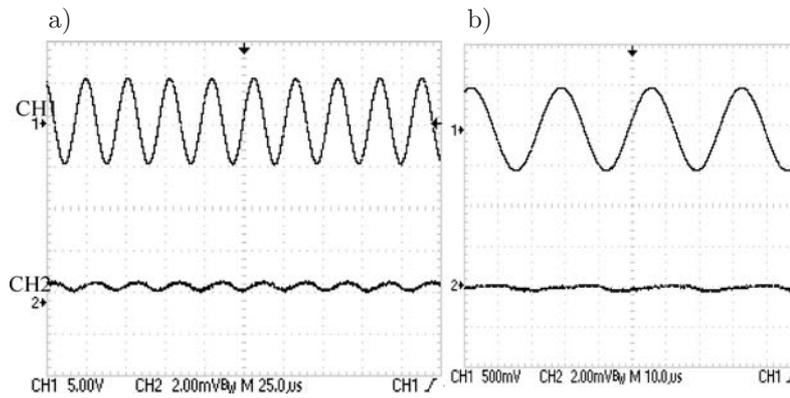
Fig. 9. Waves obtained on the oscilloscope screen for power supplied to the transducer  $P = 4 \text{ W}$ : a) without using the air gap, b) after using the air gap, CH1 is the ultrasonic input signal, and CH2 is the ultrasonic output signal (variable component of the signal).
