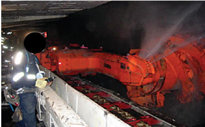
Figure 4: A view of longwall excavation with equipment during exploitation [3].
