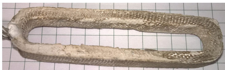
Fig. 1. HT° inorganic coil after tests at 500°C
