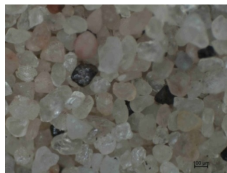
Fig. 4. Surface of the reclamation sand matrix after the thermal reclamation at 650°C (sample IV).
