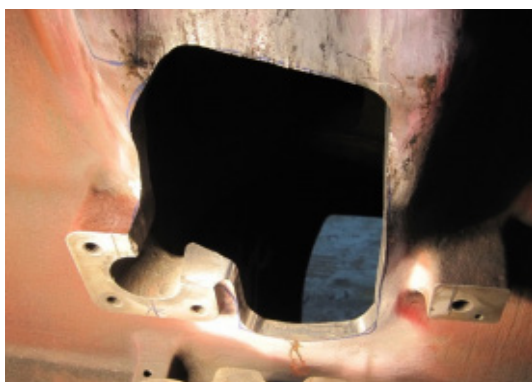
Fig. 2. Application of the laser cutting on cast iron
