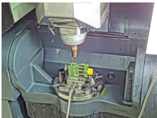
Fig. 2. Sample fixed to dynamometer on the Ultrasonic 20 Linear milling machine
