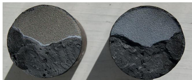
Fig. 11. Exemplary rupture of sample with coating sprayed with 97%Al 2 O 3 +3%TiO 2 powder
