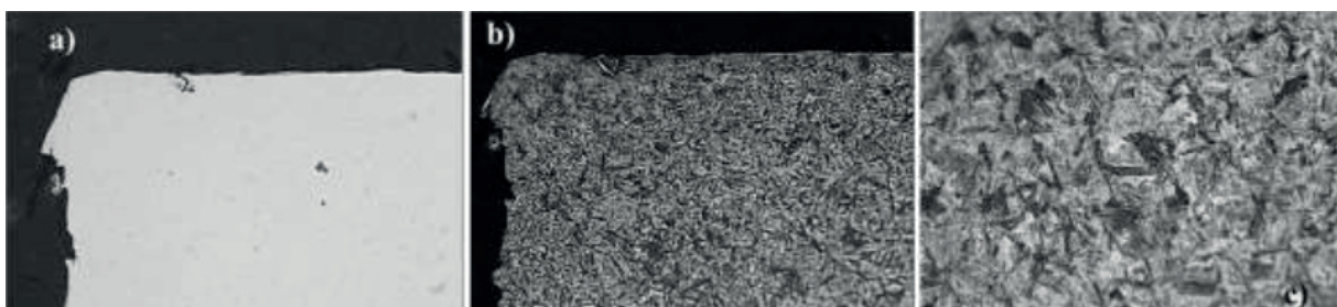
Fig. 4. Results of metallographic analysis for the stabilizer bar subjected to shot peening (Source TKF & s)
