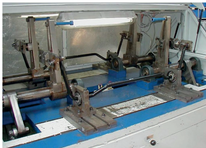
Fig. 2. Fatigue testing machine Franke 1 with 2 stabilizer bars (Source TKF & s)
