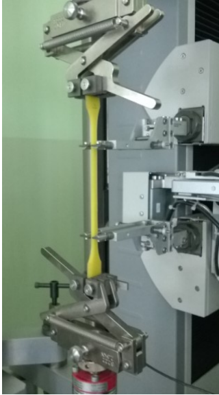
Fig. 2. The uniaxial tension test of elastomer sample
