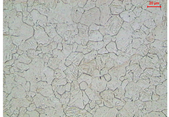
Fig. 2. Typical prior austenite microstructure of a structural steel
