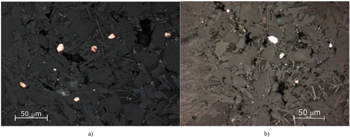
Fig. 6. Zone II: a) equiaxed structure – 800×, b) the composite structure from the zones I and II, 1000×
