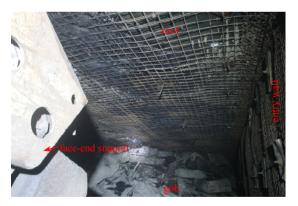
Fig. 4. Hanging roof in the end of longwall mining face
