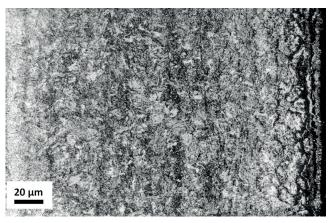
Fig. 6. The microstructure of nitrided layers of oxygen diffusion
