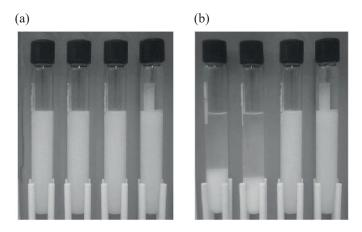
Fig. 6. Flocculation in mixtures of PA latex and inorganic salts: (a) immediately after mixing, (b) stable state (from left to right, the salts in mixture are Ca(OH)<sub>2</sub>, CaCl<sub>2</sub>, NaOH, and NaCl, respectively) [38]
