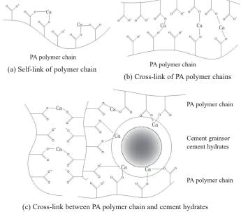
Fig. 7. Reaction between Ca<sup>2+</sup> and PA polymer chain [39]
