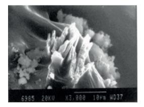
Fig. 3. Calcium acetate crystals as the product of hydrolysis of PVAc in cement paste [33]
