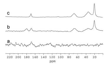
Fig. 5. SPE <sup>13</sup>C MAS NMR spectra of (a) white cement without additives after 56 days of hydration, (b) hydrated EVA/white cement after 56 days of hydration, (c) EVA [37]
