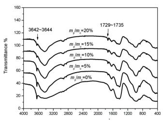
Fig. 8. FTIR spectra of cement pastes, with and without SAE powder, cured for 28 days  $(m_p/m_c \text{ is polymer/cement ratio})$  [43]
