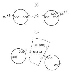
Fig. 9. Schematic illustration of cross-linking of polymer particles by (a) divalent Ca-ions and (b) Ca(OH)<sub>2</sub> solid particles [44]
