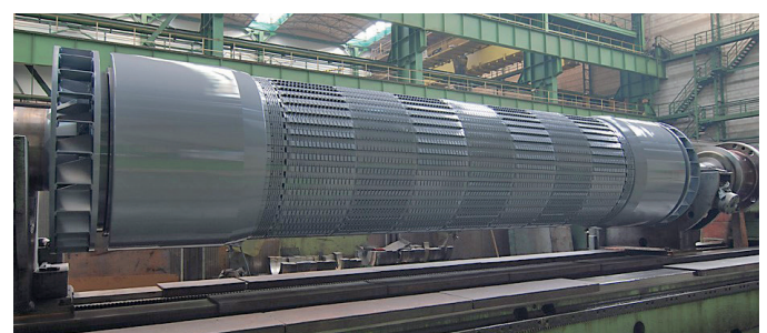
Fig. 2. New rotor enabling a rise in TWW-500-2 turbogenerator power up to 560 MW
