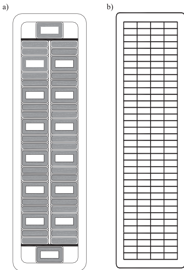
Fig. 6. Cross-section of stator bars of TGW-63 turbogenerator: a) manufacturer's design (direct cooling with distillate), b) after modernization (indirect hydrogen)
