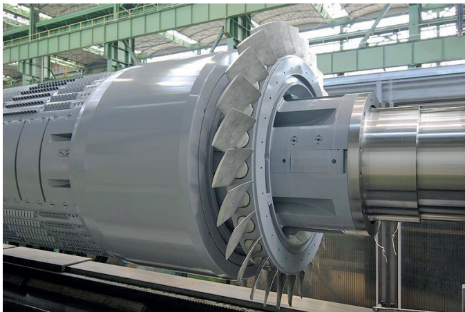
Fig. 3. Modernized rotor of TWW-320-2Y3 turbogenerator
