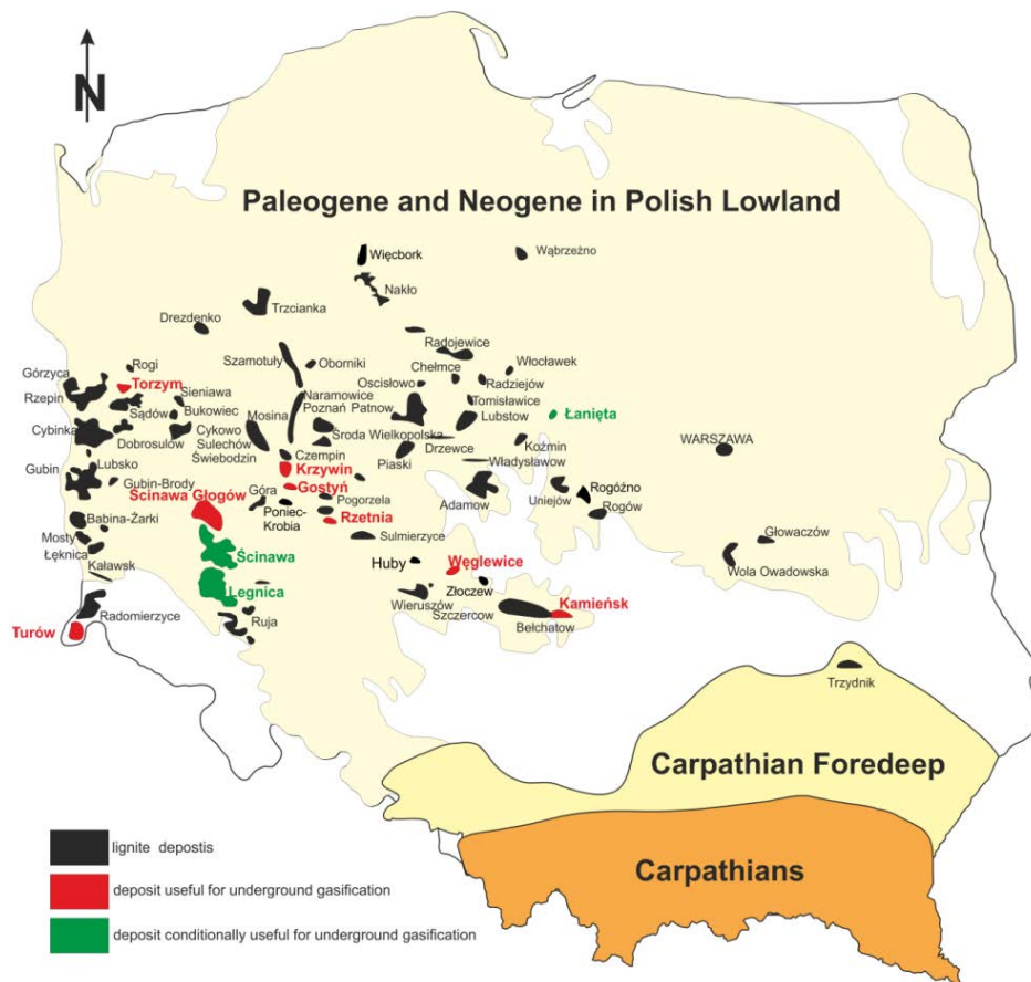
Fig. 2. Location map of lignite deposits useful for underground gasification (according to Bielowicz and Kasiński 2014 ; Matl et al. 2015 )
