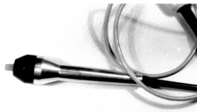
Fig. 7. A fabricated thermal sensor based on SAW.
