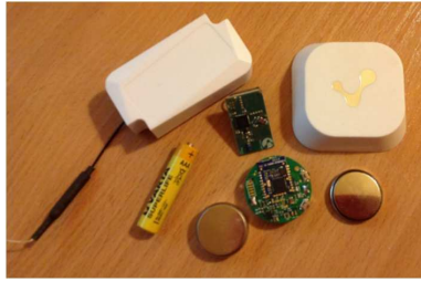
Fig. 1. Beacons used in the presented research (from left: AprilBeacon 227A, AprilBeacon sensor 401, Kontakt.io Smart Beacon).
