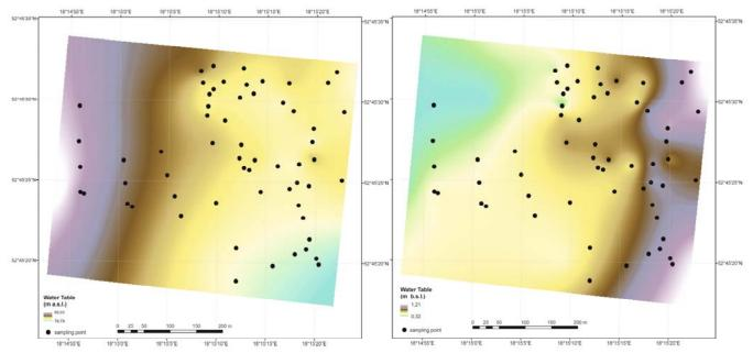
Fig. 2. Map of a hydroisohypse and hydroisobath
