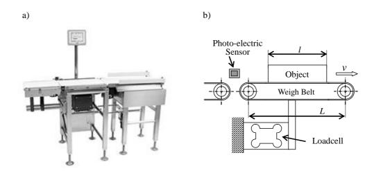
Fig. 1. a) Checkweigher and b) its devices for weighing.
