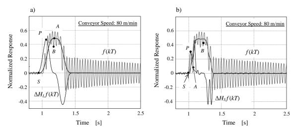
Fig. 5. Example of actual f(kT) and its derivative signals in the case that conveyor speed is 80 m/min; f(kT),  $H_L$  f(kT) and  $\Delta H_L f(kT)$  are plotted in a) and f(kT),  $H_S f(kT)$  and  $\Delta H_S f(kT)$  are plotted in b).
