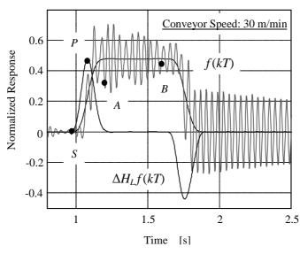
Fig. 4. Example of actual f(kT),  $H_L f(kT)$  and  $\Delta H_L f(kT)$  in the case that conveyor speed is 30 m/min.
