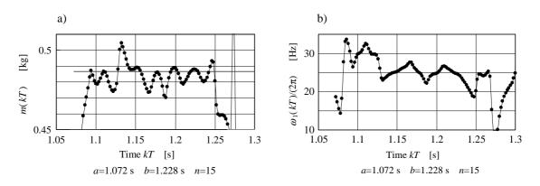
Fig. 6. Estimated values obtained by using  $G_k(z)$  designed for f(kT) in Fig. 5; a) the estimated mass of object m(kT) and b) the estimated angular frequency of dominant component  $\omega_1(kT)/(2\pi)$ .
