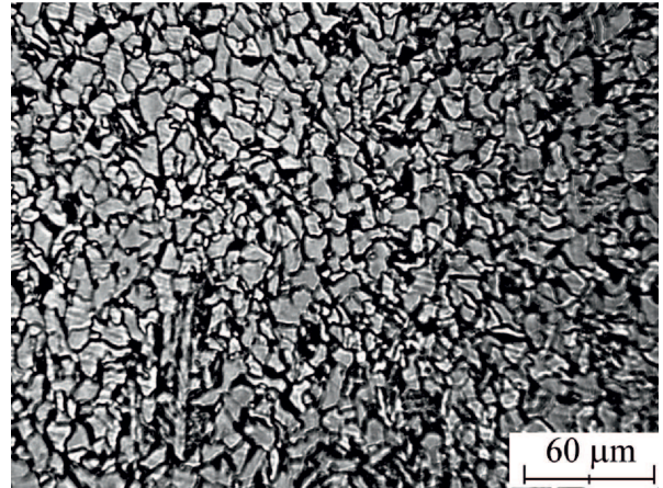
Fig. 5. The microstructure of the specimen after rolling simulation according to scheme 3 from Table 2
