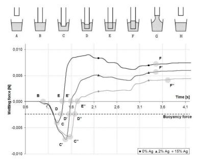
Fig. 7. The wetting force changes and specific points for Cu-based brazes with Ag addition (braze  $1 - \blacksquare$ ; braze  $2 - \blacktriangle$ ; braze  $3 - \blacklozenge$ ) within the marked area (Fig. 6).
