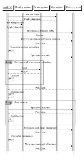
Fig. 5. A flow diagram of the measurement experiment.
