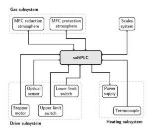
Fig. 3. The architecture of the research stand with reference to heating, gas, drive, scales subsystems and controlling devices.
