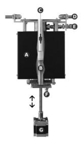
Fig. 4. A cross-section of the measurement system (A – the heating system; B – the base and the pot with a liquid braze; C – the tested specimen and its mounting; D – the specimen detection system; E, F – the gas supply system; G – the driver system).
