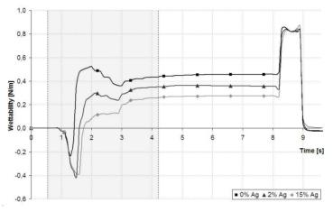
Fig. 6. The wettability changes registered for Cu-based brazes with Ag addition described above (braze  $1 - \bullet$ ; braze  $2 - \bullet$ ; braze  $3 - \bullet$ ) with an area selected for a detailed analysis of dynamics.
