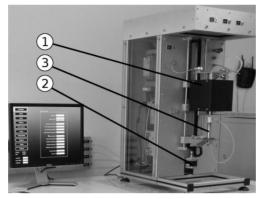
Fig. 2. An overview of the wetting force measurement system (1 – heating; 2 – driver; 3 – loading subsystems).
