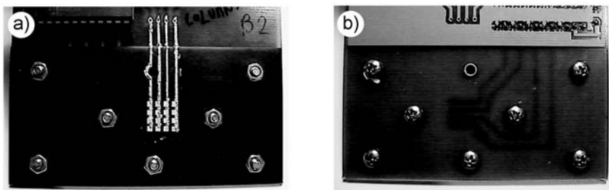
Fig. 5. Part of the designed ultrasonic matrix: a) front, b) back.
