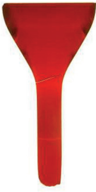
Fig. 10. Photo in transient light for a conical part of thin longitudinal \text{ZnGeP}_2 slice
