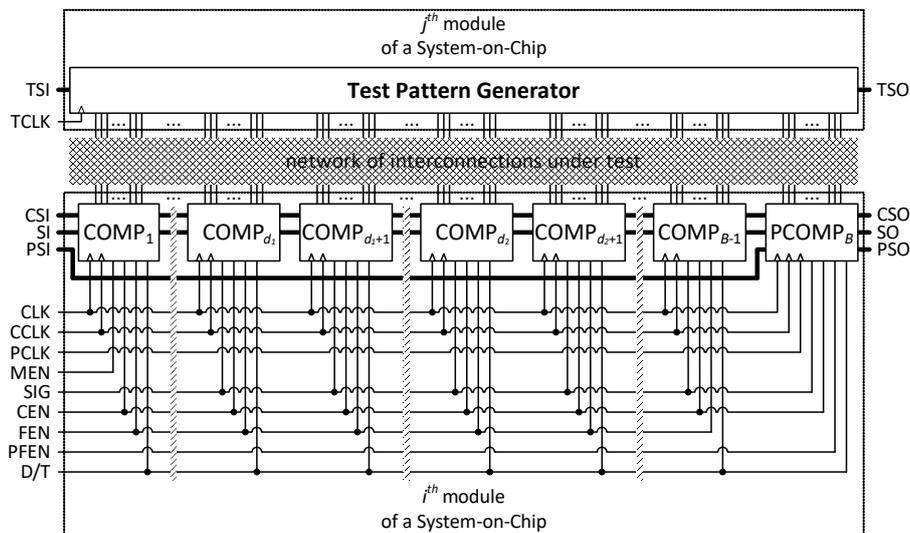
Fig. 5. Block diagram of the IBIST structure comprising a single module of the PCOMP type
