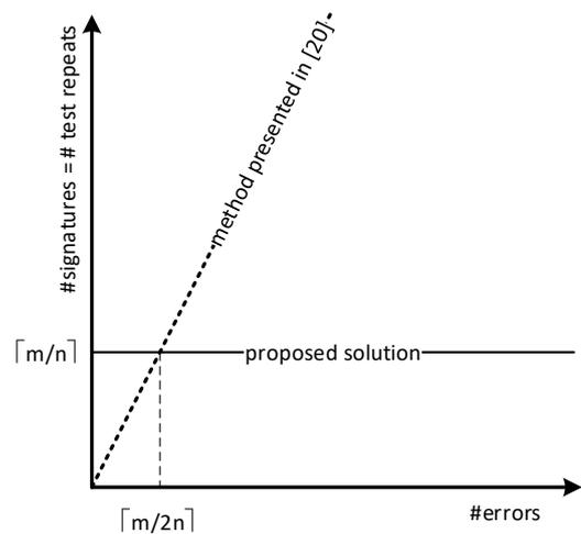
Fig. 8. Graphs illustrating the relationship between the number of  $n$ -bit signatures, which are necessary to determine  $m$ -bit sequence of the test response and the number of errors in that sequence; the graphs are presented for the method developed in [20] and the solution disclosed in [12] and in this article
