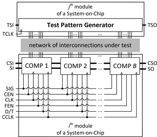
Fig. 1. Block diagram of the hardware used to test the network of connections between the digital cores of a system-on-chip
