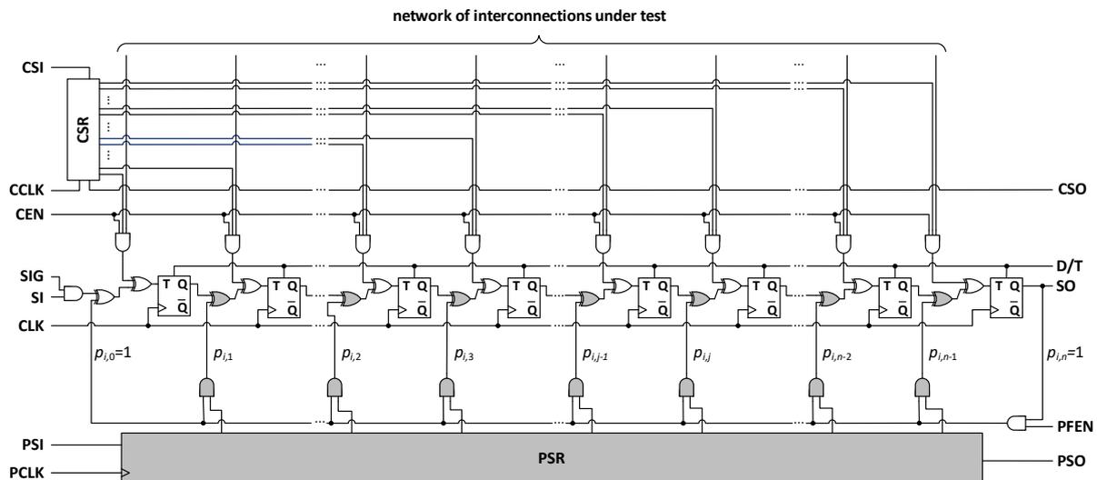
Fig. 4. Scheme of the PCOMP module
