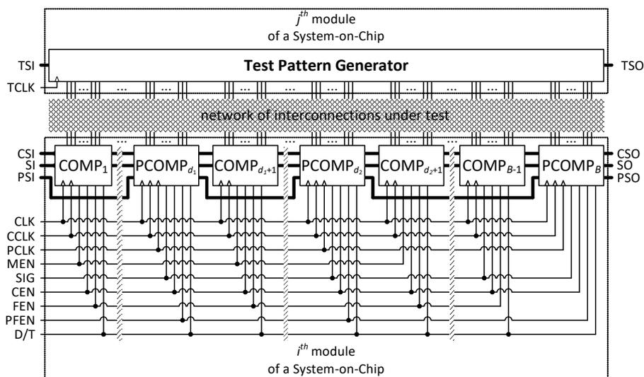
Fig. 7. Block diagram of the IBIST structure comprising D = 3 modules of the PCOMP type
