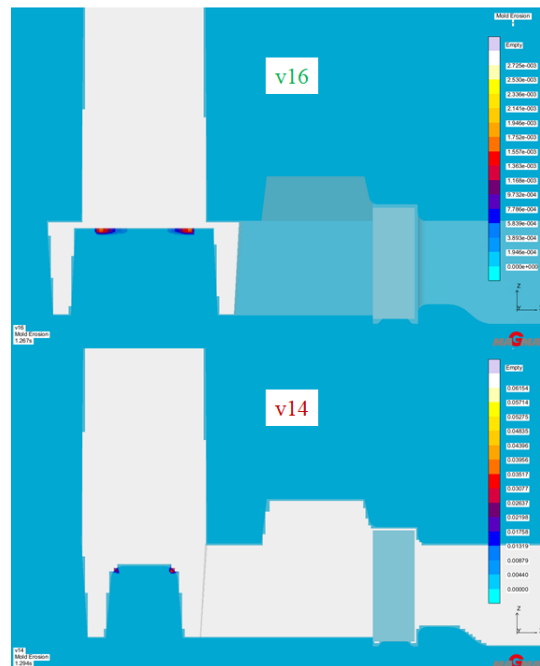
Fig. 11. Mould erosion comparison – best version v16, worst v14
