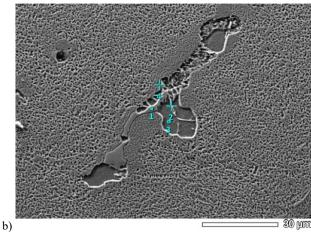
Fig. 5. The microstructure of the IN 713C with the  $(\gamma + \gamma')$  eutectic islands: a) LM, b) SEM
