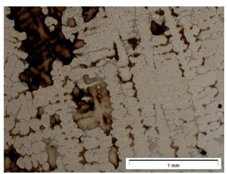
Fig. 1. Microstructure of IN 713C alloy in the as-cast condition; LM
