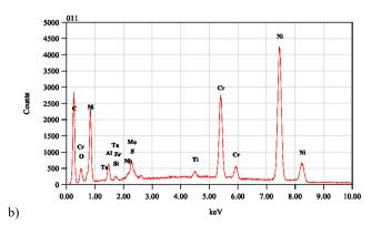
Fig. 6. a) The crack identified in the structure of the pad weld, b) The chemical composition of the crack
