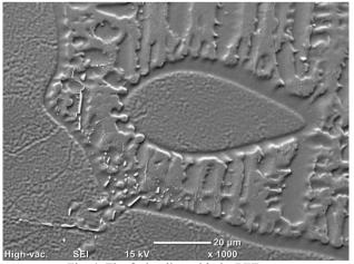
Fig. 4. The fusion line with the PFZ area
