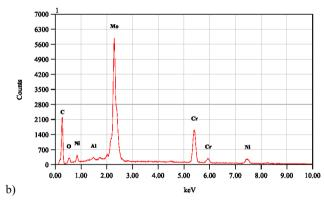
Fig. 3. a) The Cr and Mo- enriched carbide particles, b) The chemical composition of Cr and Mo- enriched carbide particles
