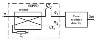
Fig. 8. A block diagram of a "sine" type frequency detector.
