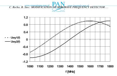
Fig. 7. Characteristics of input voltage for a "cosine" type SFD operating in a range of 1–1.8 GHz without a phase shifter and with a phase shifter with a shift of 45 degrees for n = 1 (solid line – a curve of SFD output voltage with a phase shifter, dashed line – a curve of output voltage without a phase shifter –).
