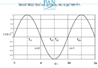
Fig. 9. Ranges of an unambiguous reading of frequencies for a "sine" type detector of frequency.
