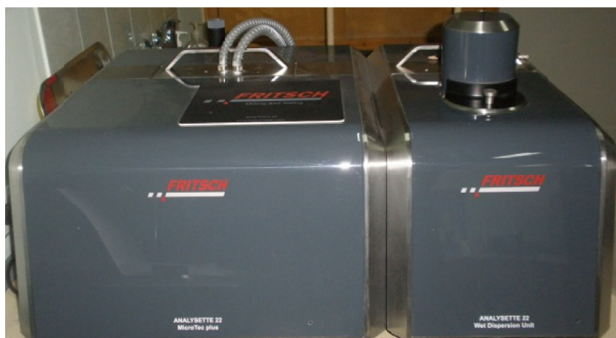
Fig. 3. Laser instrument for measurement of particles – type „Analysette 22 MicroTec Plus
