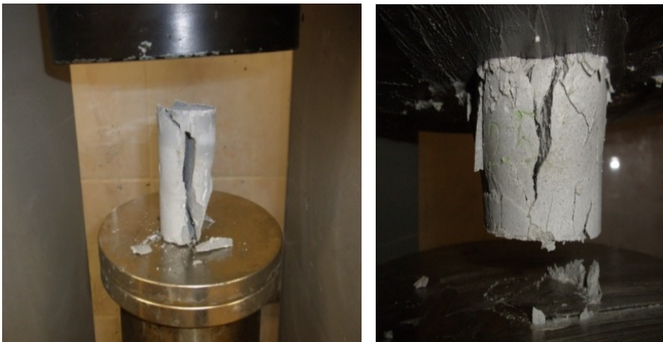
Fig. 11. Examples of samples after compressive strength tests
