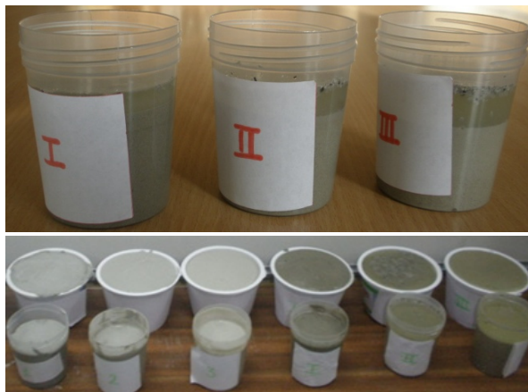
Fig. 6. Samples of waste mixtures, type B, with redundant water (above), and without the redundant water, type A (below)
