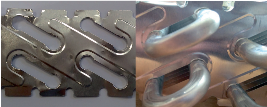
Figure 2: Geometry of egg-crate type heat exchanger: plate fin on the left, plate fin tube assembly on the right.
